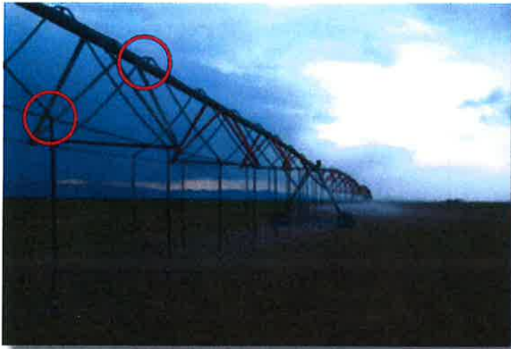
Figure 1. Double goosenecks (upper circle) and truss-rod hose clamps (lower circle) used to decrease the drop spacing and increase the number of drops. Photo by Howard Neibling, University of Idaho.
