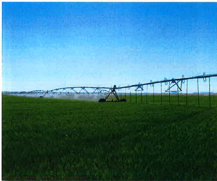
Figure 2. LESA span (left) and conventional span (right) 2014 Mark Telford spring wheat, Arco. Photo by Howard Neibling, University of Idaho.
